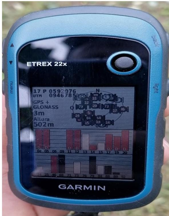
**Figura 2** GPS satelital “GARMIN ETREX 22X”.
